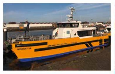
The Windcat MK3.2XL offers the same large and comfortable accommodation as the standard MK3 vessels, however, with the advantage of a raised wheelhouse and a much larger foredeck. After the lengthening of the vessel, the Windcat 34XL offers a 49m² fore deck, which provides space for a standard 10 foot container as well as additional cargo.
